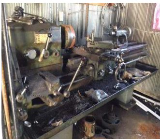
Woodhouse metal Lathe with 5-foot bed
