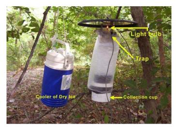
If you see a device like the one pictured in the woods, don't disturb it. It's a mosquito trap used by the Wahta Mohawks to collect samples as part of its surveillance of West Nile Virus in the community. Traps have been set up in 4 locations, evenly spaced throughout the area. They are mostly off the beaten path in wooded areas. We do move the traps around sometimes. Traps are checked and emptied weekly.
